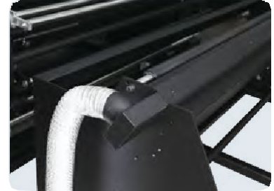
Fume extraction unit
