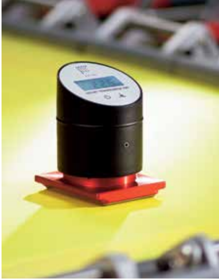
Checking the mesh tension with SEFAR® Tensocheck 100: Equal high tension, less tension loss than conventional meshes
