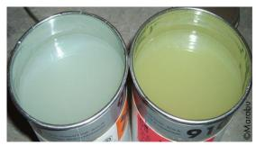
The separation of these individual components, however, may affect the optical appearance in a similar way. Therefore, it is necessary to stir the ink homogeneously, and to evaluate the printed colour proof.
